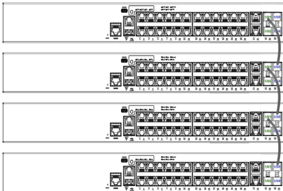
FIGURE 10 ICX 7150 24-port model, linear stack
