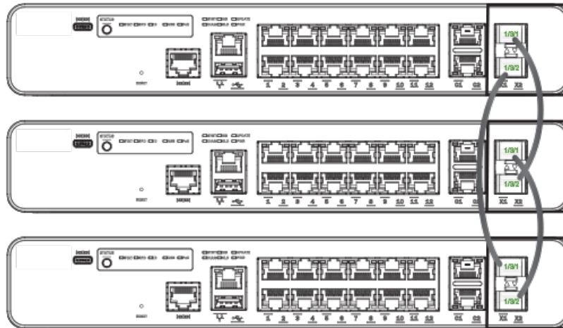
FIGURE 9 ICX 7150-C12P stack ring topology
