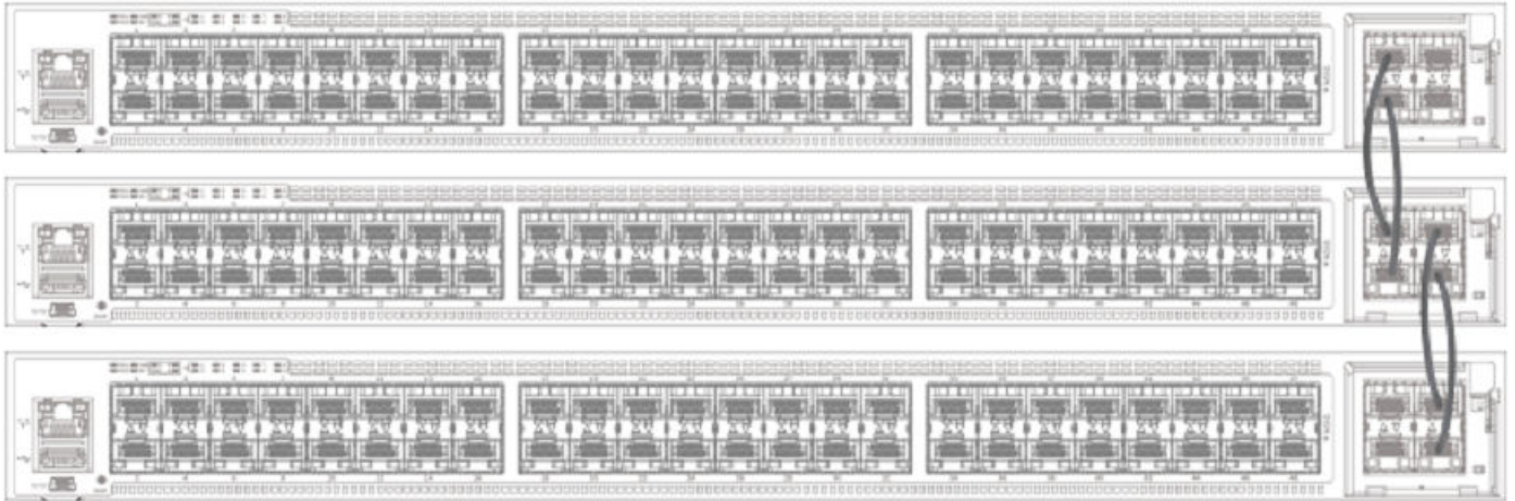
FIGURE 22 ICX 7450 4 X 10-Gbps linear stack
