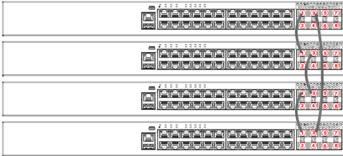
FIGURE 16 ICX 7250-24P ring stack
