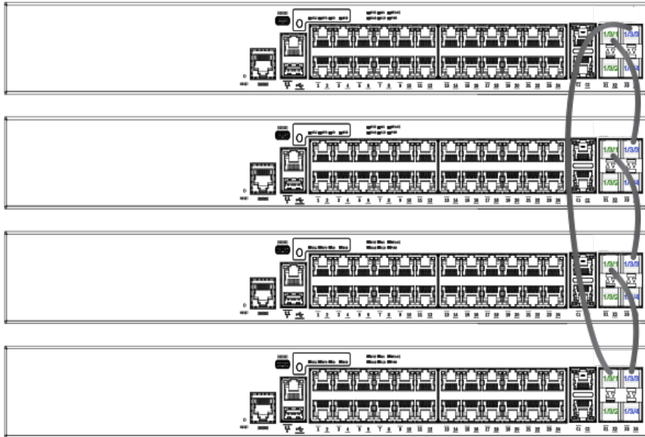
FIGURE 11 ICX 7150 24-port stack ring topology
